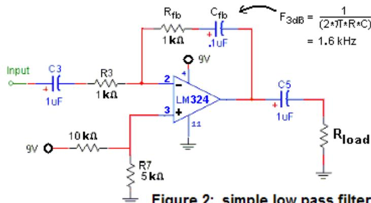
**Figure 2: simple low pass filter**
