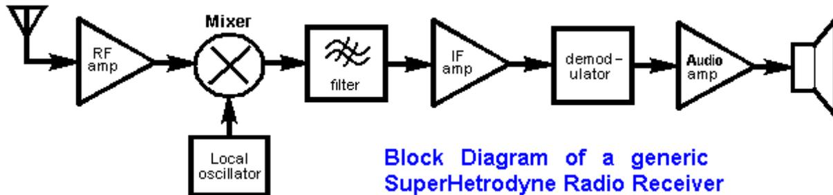
Block Diagram of a generic SuperHetrodyne Radio Receiver
